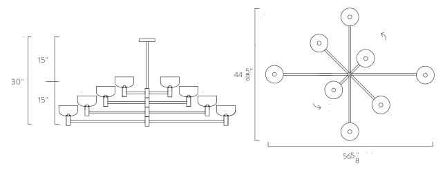
Otto Luce has a solid milled and tubular brass armature with handblown gilded glass shades for atmospheric light. Arms rotate into position from center axis.
